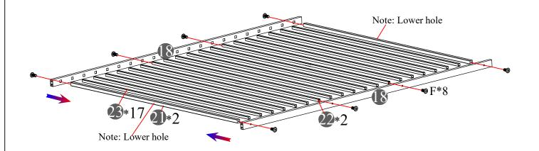
NOTE: In this step, DO NOT tighten any bolt until you connect all part together.
