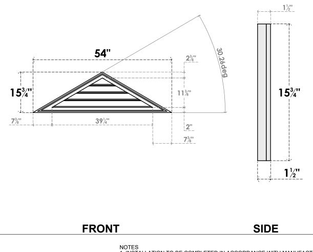
1. INSTALLATION TO BE COMPLETED IN ACCORDANCE WITH MANUFACTURER'S SPECIFICATIONS. 2. DRAWING MAY NOT BE TO SCALE
