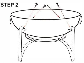
Align the holes in Fire Bowl (A) with the holes on the top of Legs (B). Hand-tighten 4x Bolts (G). Tighten all bolts with a Phillips screwdriver (not included).
