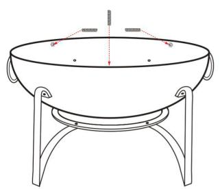
Hand-tighten 3x Grub Screws (F) to the inside rim of Fire Bowl (A). DO NOT use tools to tighten the grub screws.
