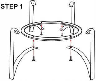
Align the holes on Legs (B) with the holes on Support Ring (C) and hand-tighten 4x Bolts (G).
