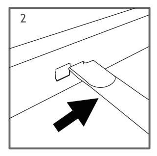
1.Insert slats into the hole on sidebar in the correct orientation. 2. Push the slats into the gaps.
