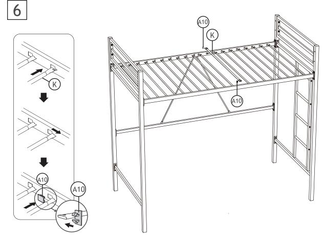
**Notice:**Pay attention to the direction of the buckles(A10). The convex side of the buckle faces into the bar(K).
