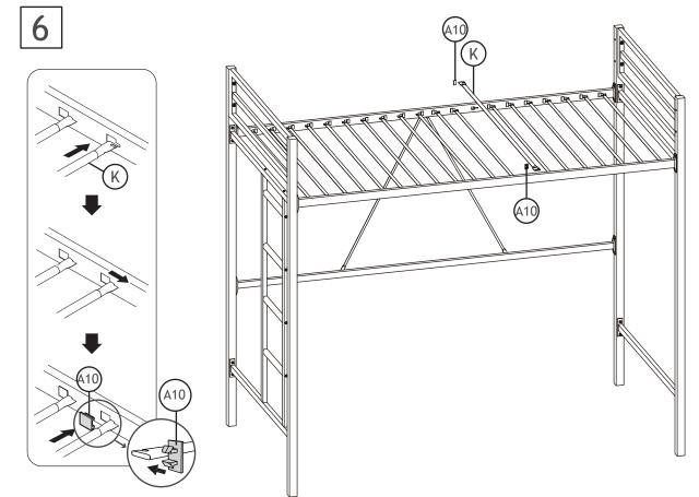
**Notice:**Pay attention to the direction of the buckles(A10). The convex side of the buckle faces into the bar(K).
