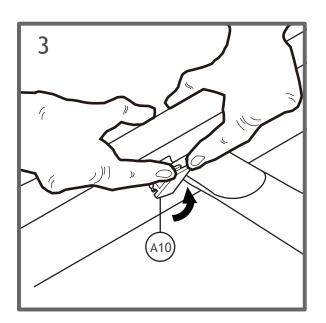
3.Put the plastic clamp intothe lower part of the hole on45 degree.
