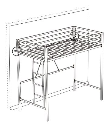
Tie the bunk bed with F3. Screw F2 through the holes of F3 and then into F1.
