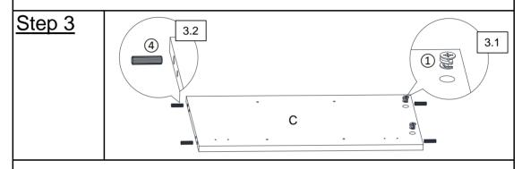
**3.1)** Insert Cam Locks(①) into mounting positions on Right Side Panel(C) by hand.
