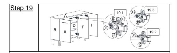
**19.1)** Attach Connectors((10)) to Left Side Panel(B), Right Side Panel(C) and Center Panel(D) with Screws((6)) using Screwdriver((13)).
