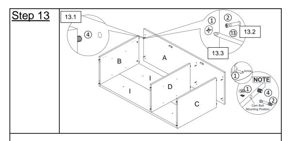
**13.1)** Insert Positioning Dowels(④) from Left Side Panel(B), Right Side Panel(C) and Center Panel(D) into mounting positions on Top Panel(A).
