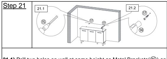
**21.1)** Drill two holes on wall at same height as Metal Brackets(16) on Shoe Cabinet with Power Drill(15).
