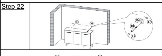
Attach Metal Brackets(((16)) to Wall Plugs(((17)) using Wall Plug Screws(((18)) with Screwdriver(((13)).
