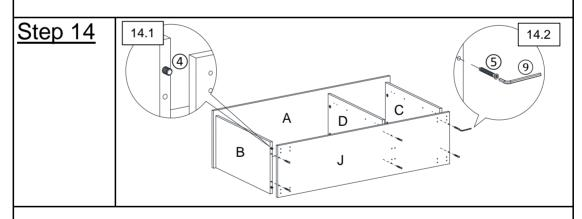
**14.1)** Insert Positioning Dowels(④) from Left Side Panel(B), Right Side Panel(C) and Center Panel(D) into mounting positions on Bottom Panel(J).
