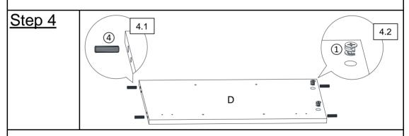
**4.1)** Insert Cam Locks(①) into mounting positions on Center Panel(D) by hand.
