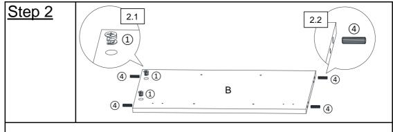
**2.1)** Insert Cam Locks(①) into mounting positions on Left Side Panel(B) by hand.
