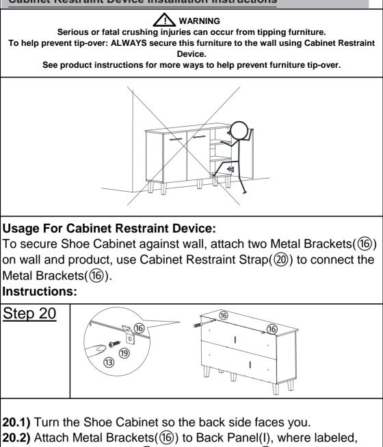
using Pan Head Screws((19)) with Screwdriver((13)).
