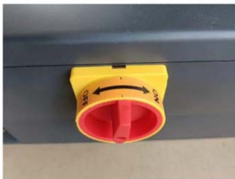
A. The power switch rotates clockwise. ON-Turn on OFF-Turn off
