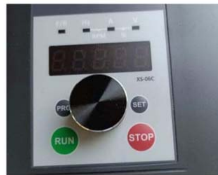
B. Controller panel operating instructions RUN-Run button STOP stop button
