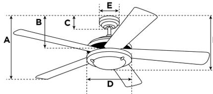
If a Combo Style Fan with a 4" Down Rod is installed without the Down Rod, Subtract 3" from the Dimensions Listed (A, B, F).
