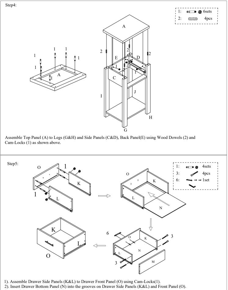
3). Attach Drawer Back Panel (M) to Drawer Side Panels (K&L) using Bolts (3).
