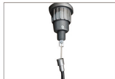
03. Use fingernall to pull out the bead from the drive line and insert it into the white hose
