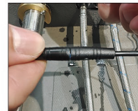
04. Connect the electricity line with motor
