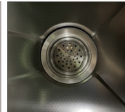
03. Use the tool to fasten the up & bottom strainer part and put the filler in
