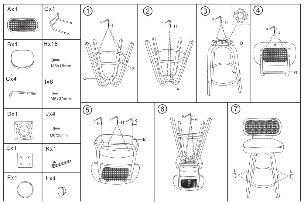
Please do not tighten the screws until the installation is complete! Thank you!
