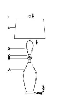
Step 1 Insert the Harp (D) into the Saddle (B). Put the shade(E) on the Harp(D), then tighten the Finial (F)into the Harp (D)
