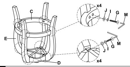
Take the Allen Wrench, and turn the bolts until the legs are secured. DO NOT TIGHTEN COMPLETELY. Stop when you feel you are adding force to tighten the bolt.
