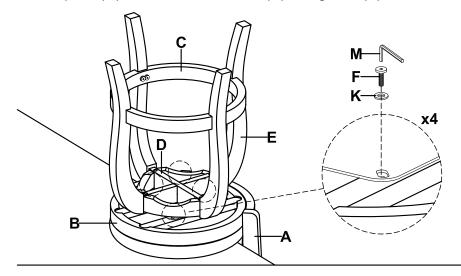
Stand the chair on an even surface and check for balance. If it wobbles, apply downward pressure on the uneven leg and tighten the bolts. Once the chair is balanced, apply pressure evenly to the center and tighten all bolts, ensuring not to over-tighten beyond the hole depth.
