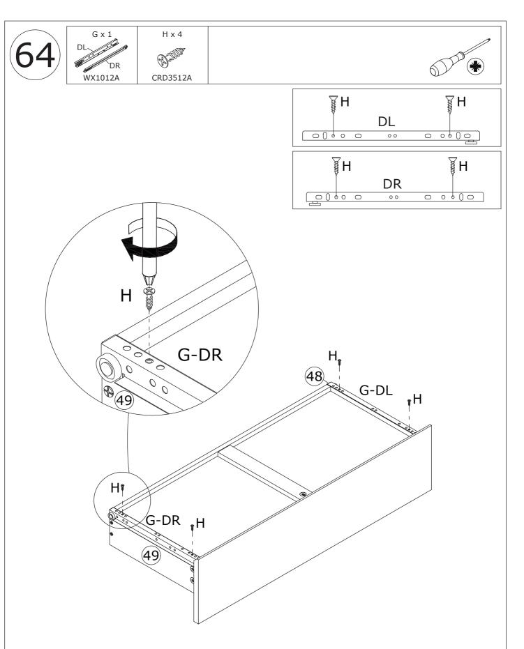
As shown in the figure, use screws (H) to fix the slide rails (G-DR, G-DL) to Panel 48 and 49.
