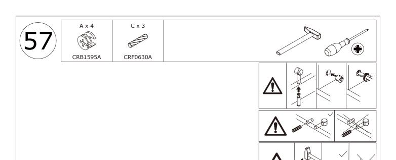
As shown in the figure, use the wooden dowels (C) to connect Panel 1 to the assembled unit, insert the eccentric wheel (A), and tighten it by rotating clockwise.
