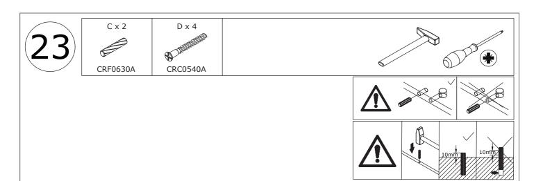
As shown in the figure, use the wooden dowels (C) to connect Panel 14 and 13 to Panel 23, and then fix them with screws (D).
