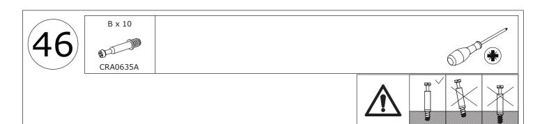
As shown in the figure, screw the self-tapping rod (B) into Panel 8.
