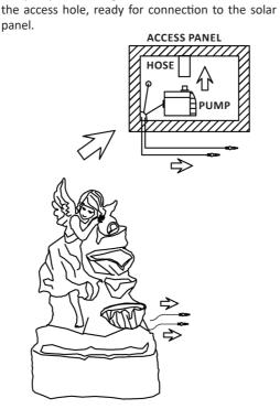
**2.** Attach the pump to the hose from the access panel on the back of the fountain body. The LED
