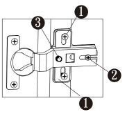
djust the cabinet door up and down adjust screw  $\,\,$  NO. 1
