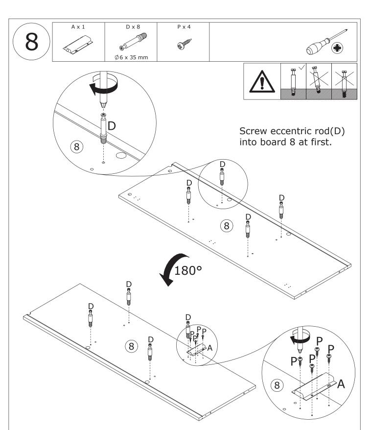
Flip to back, screw eccentric rod(D) into and fix part(A) with screw(P) as shown.
