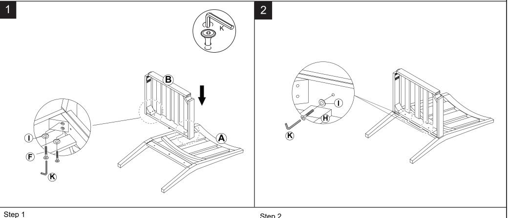
Attach Frame back (A) to Frame Seat (B) ,use Bolt (F) and Washer (I) tighten with allen key (K).
