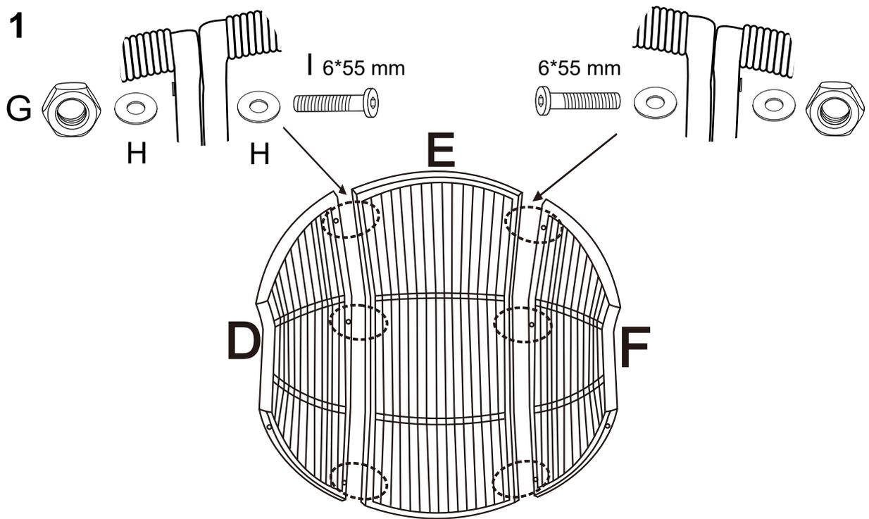
Connect right back panel (Part D) and middle back panel (Part E) with I, H and G.
