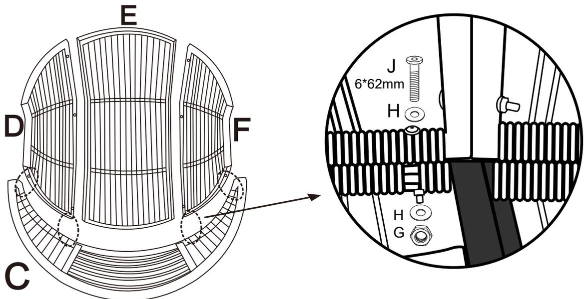
Buckle the back parts upside down on the floor.
