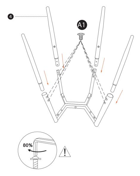
Step 3: Connect the Foot Ring to the Frame with Screw. Then Tighten Them By 80%. Make Sure the Frame is Leveled On the Ground. Then Tighten All the Screw by 100%.
