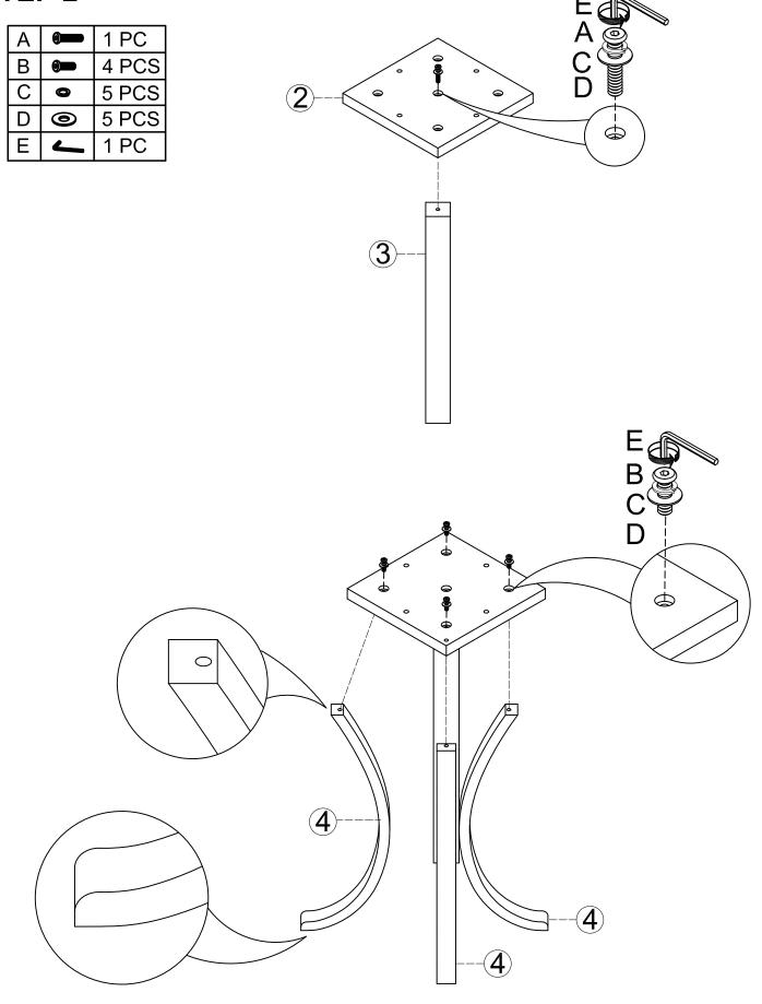
AFTER ALL LEGS ARE ALIGN WITH THE POST, TIGHTEN THE BOLTS.
