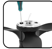
5 Rotate the lamp plate to position screw hole of each blade in turn and tighten blades with screws.
