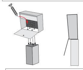
Secure the Metro to the post using a 1/2" drive socket or a 1/2" wrench.
