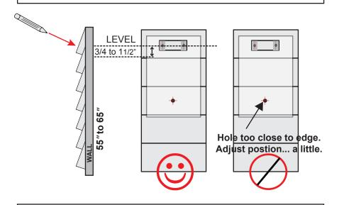
2 Using a <sup>1</sup>/8" drill bit, drill the top two pilot holes approximately 2"deep into the the wall material. Attach the mounting bracket using the two 2<sup>1</sup>/4"screws provided. Be sure to put some water resistant caulk into the holes. Now hang the Metro from the brackets shown and mark the bottom three holes with a pencil.
