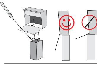
2 Using a  $^{1}/_{4}$ " drill bit, drill four pilot holes in the marked positions approximately  $^{11}/_{2}$ " deep into the wood. Attach the Metro to the post using four  $^{11}/_{2}$ " lag screws. A  $^{1}/_{2}$ " drive socket or a  $^{1}/_{2}$ " wrench may be used.
