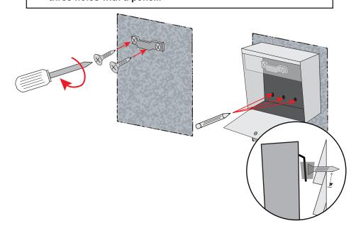
3 Using a masonry style drill bit(not provided), drill the bottom three pilot holes approximately 2"deep into the wall material. Now hang the Metro from the mounting bracket and secure to bottom using the three 21/4"screws provided. Be sure to put some weather resistant caulk into the holes. If your wall is a thick brick, stucco or concrete you may need masonry screws or anchors for attachment. Consult a contractor if necessary.
