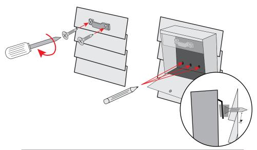
3 Using a 1/8" drill bit, drill the bottom three pilot holes approximately 2" deep into the wall material. Now hangy our Metro from the the mounting bracket. If there is a large gap between the Metro and the wall insert a bushing on the screw. Insert some water resistant caulk into the hole and secure to bottom using the remaining three 21/4" screws provided.
