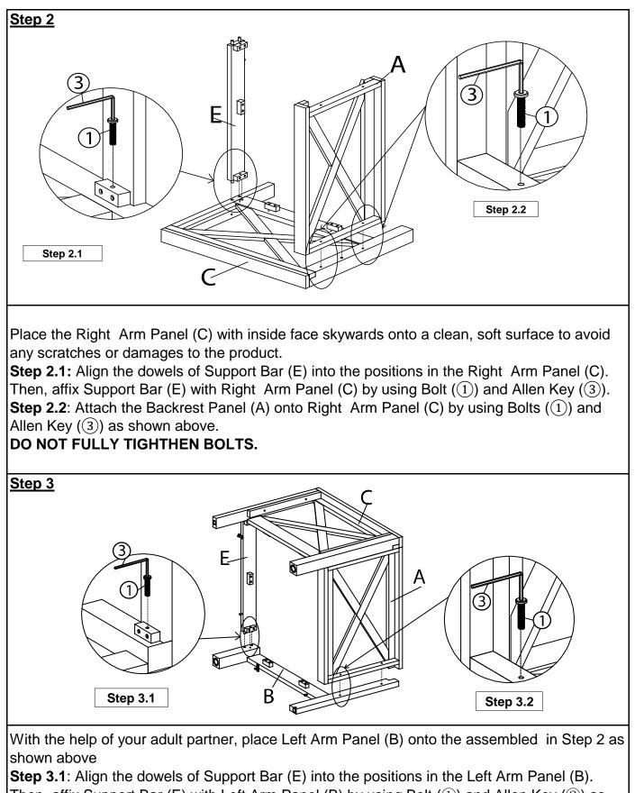
Then, affix Support Bar (E) with Left Arm Panel (B) by using Bolt (1) and Allen Key (3) as shown above.
