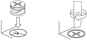
Turn the cam lock clockwise to tighten.
