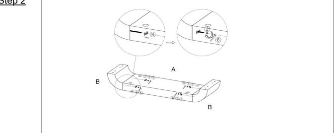
Attach the Connecting Planel(B) to Table Top(A) with Crescent Nut(③),Nut(②) using Wrench(⑥).
