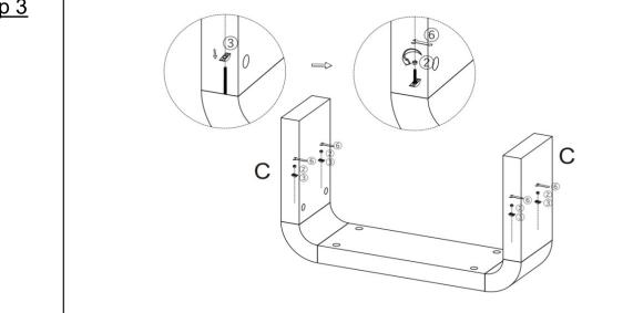
Attach the Leg(C) to Connecting Planel(B) with Crescent Nut(③),Nut(②) using Wrench(⑥).
