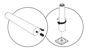
Prepare leg No.5. Remove the screw protector. Insert the screw and tighten the leg by turning it clockwise.
