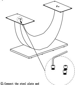
4. Place the table on the steel plate, and connect the steel plate with tabletop.
