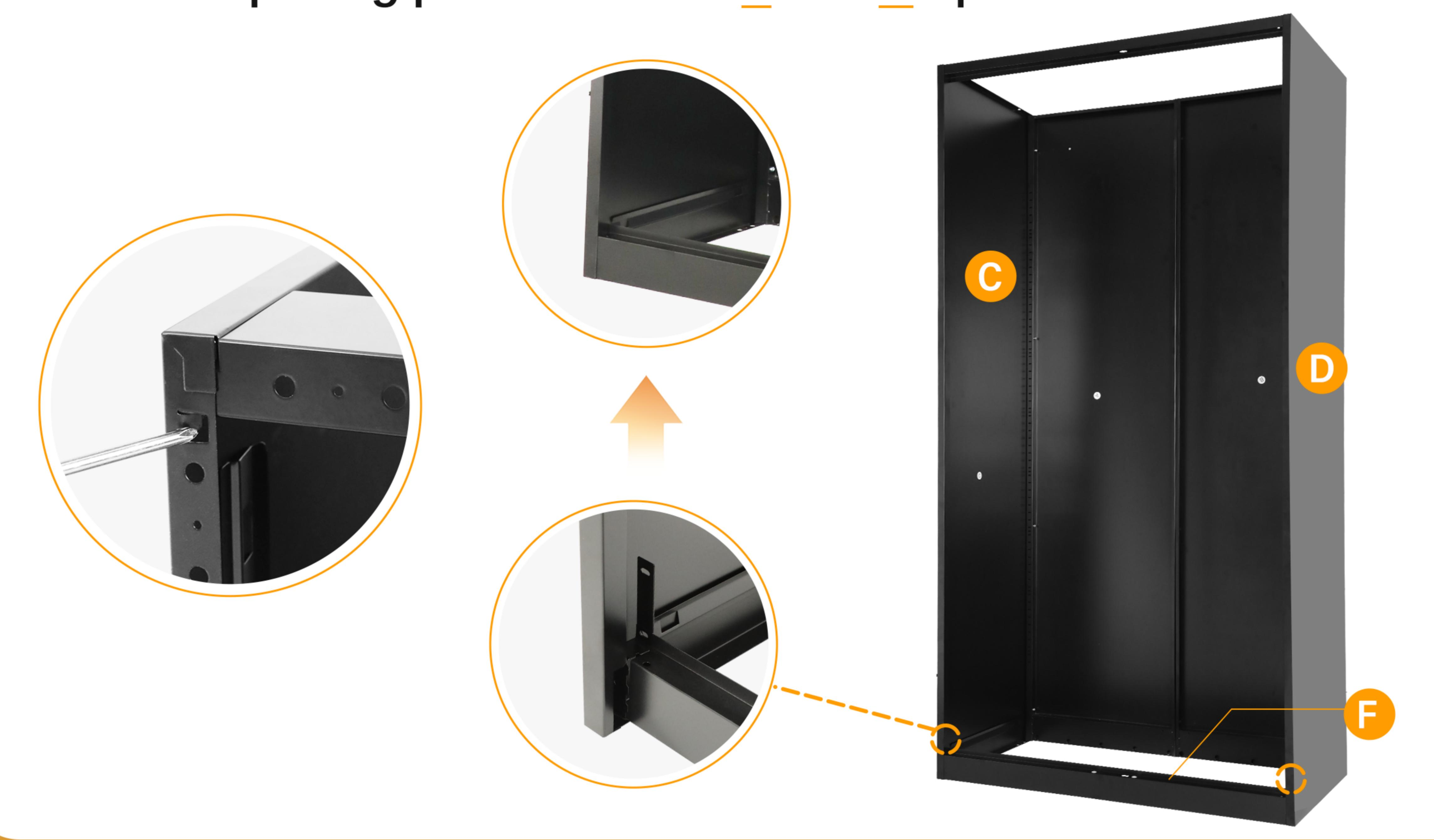
Connect C to F and D to F with four screws L.
