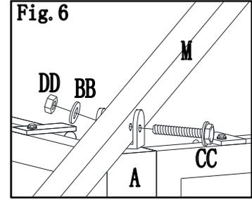
Fig.6 Attach the assembled slanting beam bottomend (M) to plate top of post(A), by using bolt(CC),washer (BB) and nut(DD).
