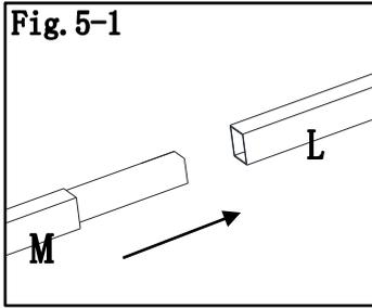
Fig.5- 1:Insert slanting bottom tube(M) into slanting beam(L).
