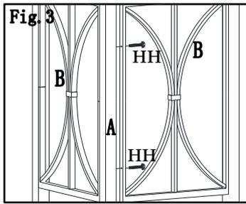
Fig.3: Attach fence(B) to post(A),by using bolt (HH).
