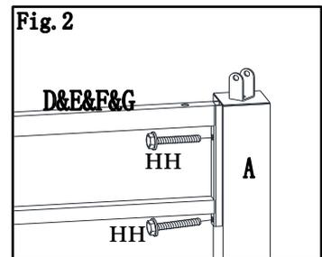
Fig.2: By using bolt(HH) fix screen to post(A).
