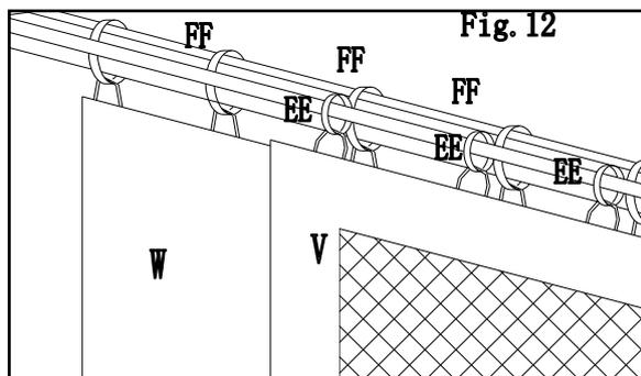
Fig.12:Using small ring (EE) hang mosquito netting (V) on netting rod (H/I) . using large ring (FF) hang curtain (W) on screen upper rod(D/E/F/G).
