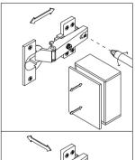
If the hinge holes are notaligned, you can tryadjusting the front and rear hinges.
