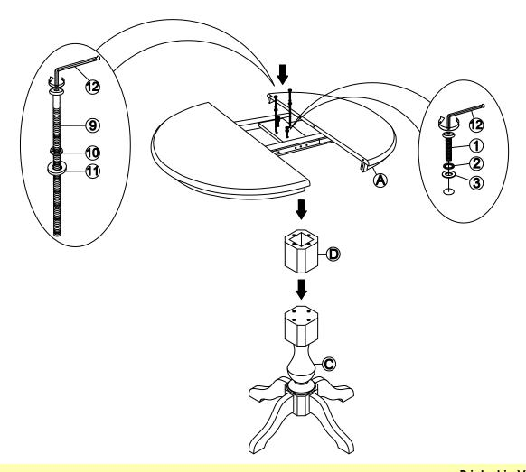
Attach mounting plate and pedestal extension (D) to the column (C) with long bolts (9), short bolts (1), washers (2), (4), (10) and (11) as shown below. Tighten with Allen key (12).
