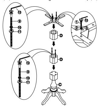
Attach the top (A) and pedestal extension (D) to the column (C) with long bolts (9), short bolts (1), washers (2), (3), (10) and (11) as shown below. Tighten with Allen key (12).
