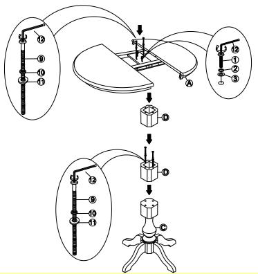
Attach mounting plate and pedestal extension (D) to the column (C) with long bolts (9), short bolts (1), washers (2), (4), (10) and (11) as shown below. Tighten with Allen key (12).
