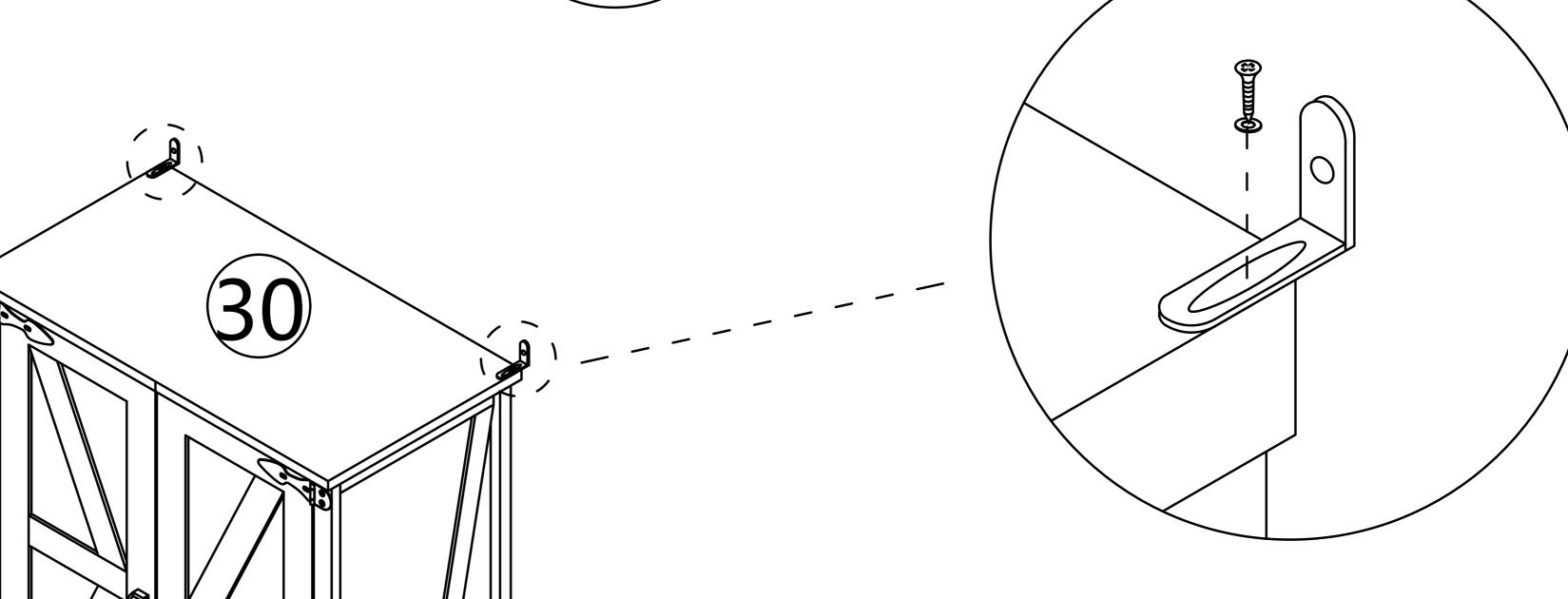
Install the anti fall hardware on the cabinet as shown in the picture first
