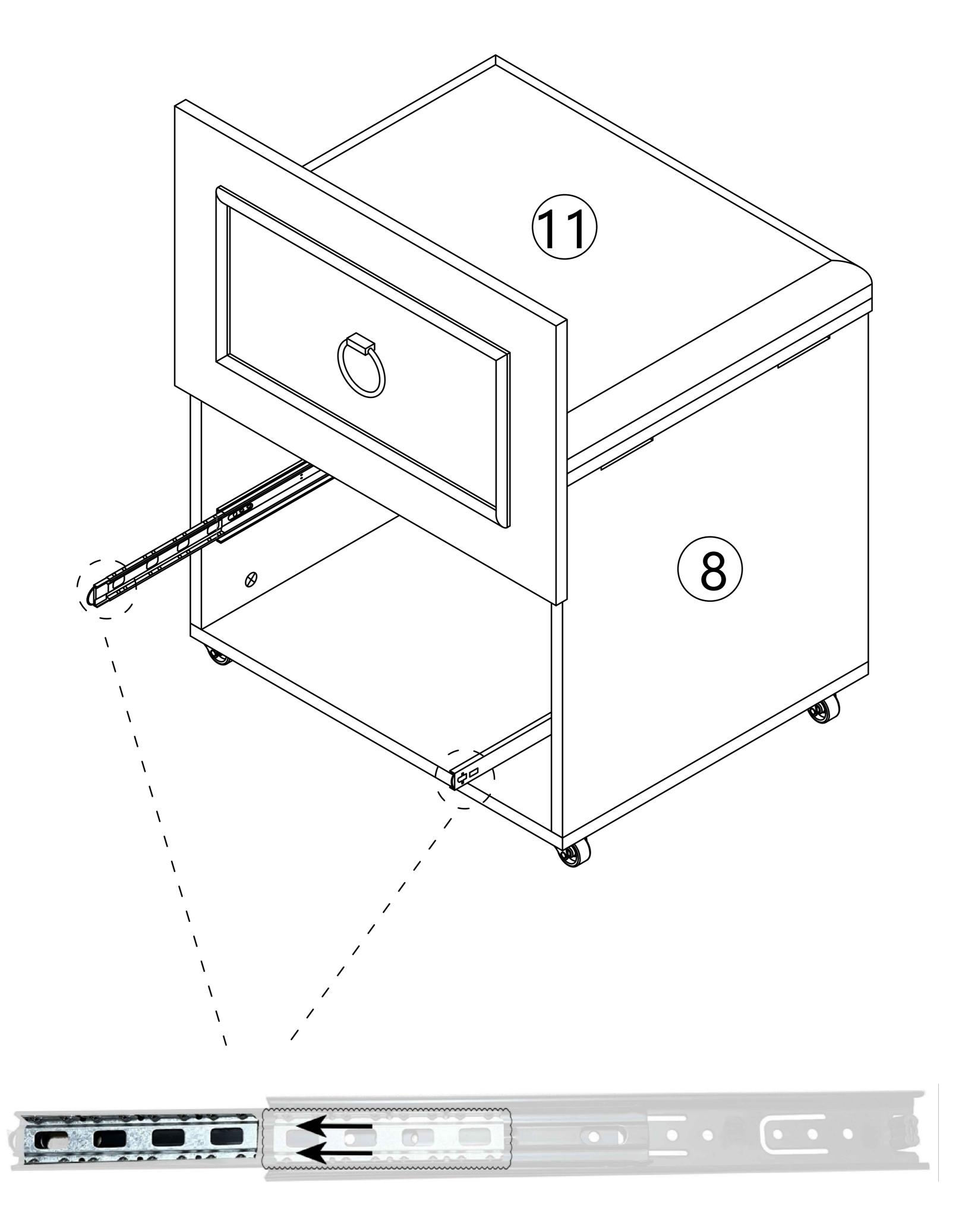
As shown, When installing the drawer, pull the guide rail out first, Slide beads are also pulled out.
