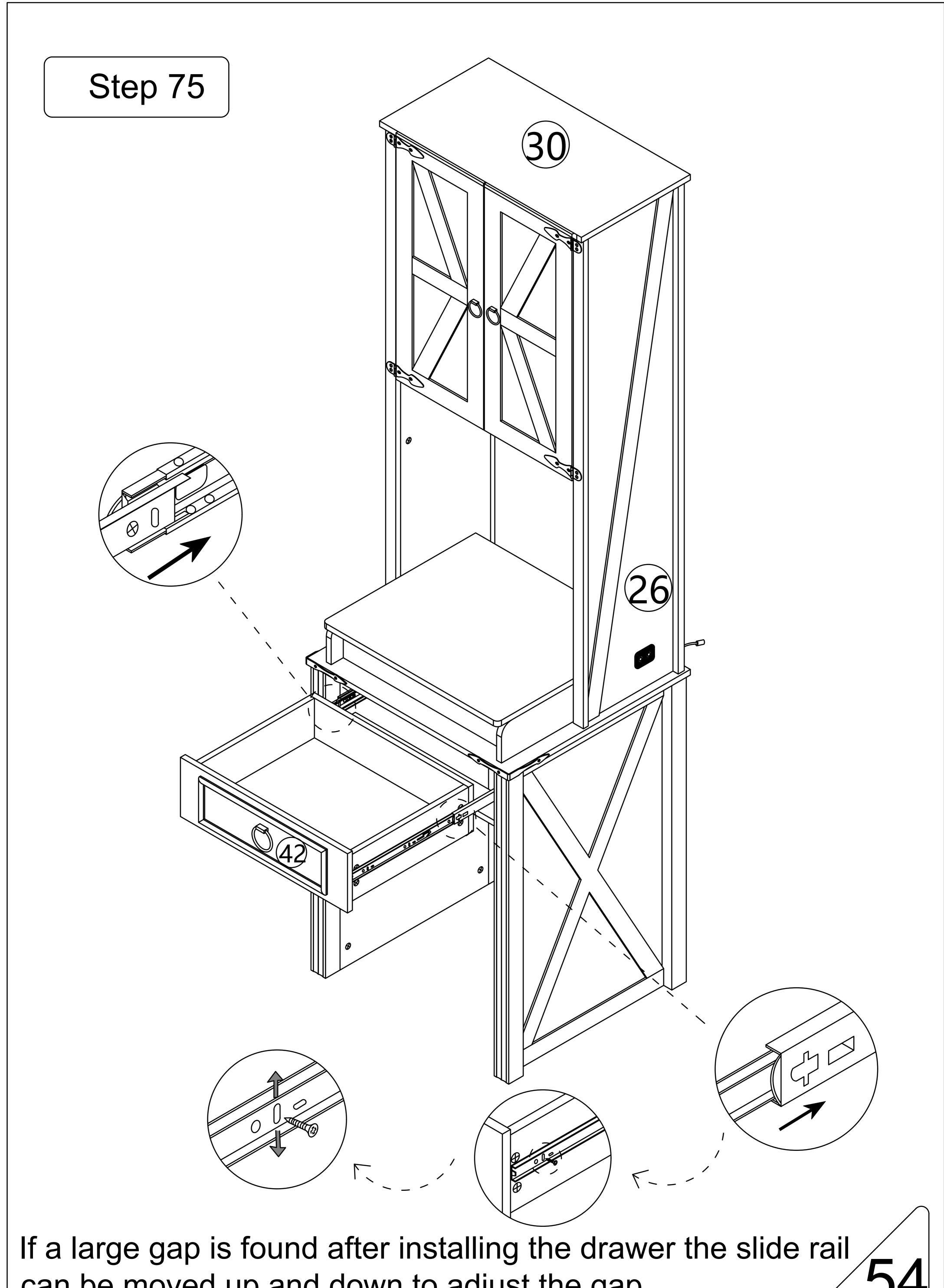
can be moved up and down to adjust the gap
