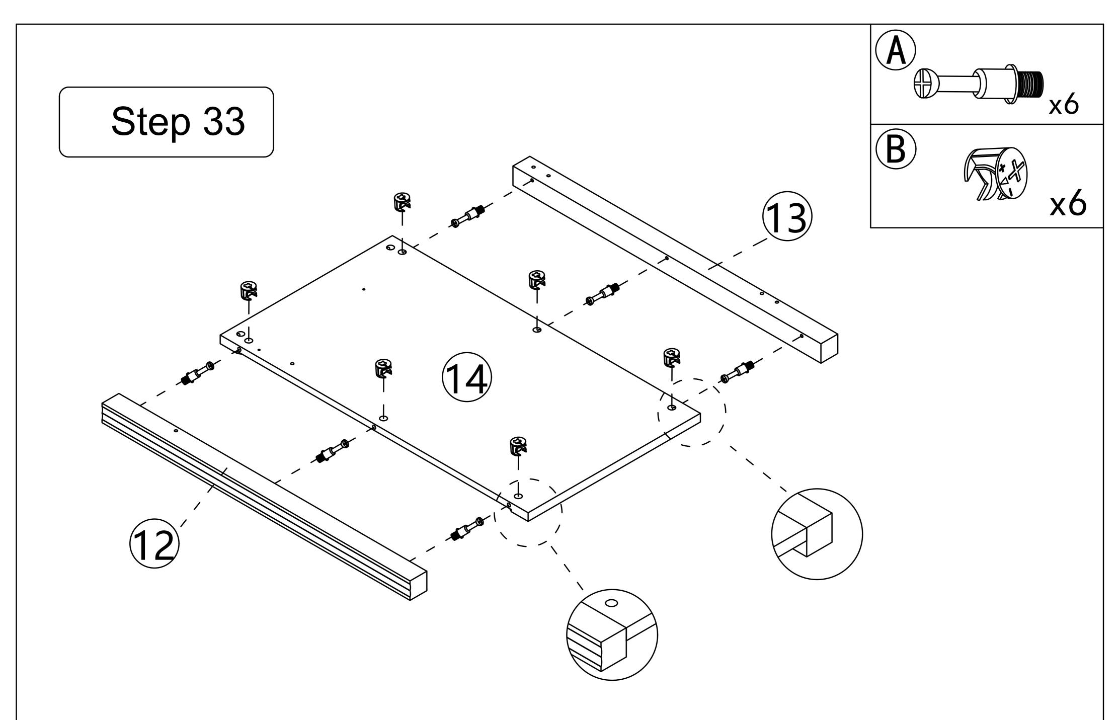
Attention: First install the two in one, then install the nut
