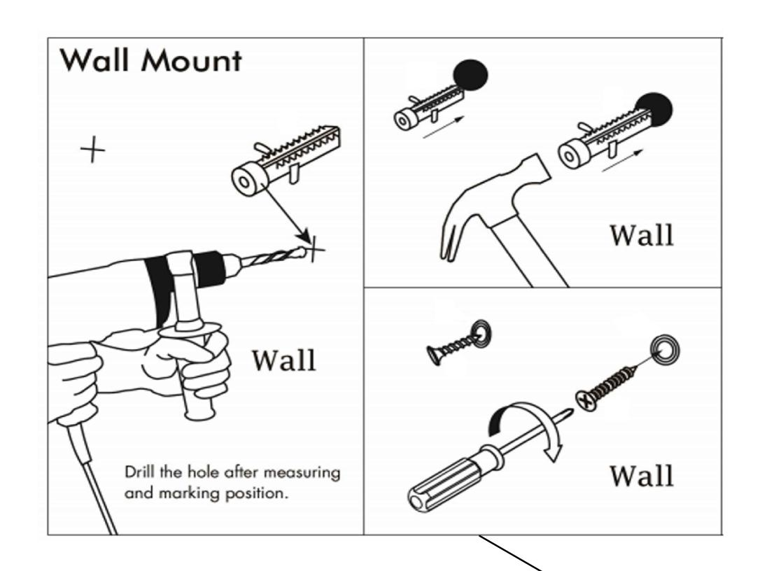
Drill the hole with an electric drill and punch in the colloidal particles
