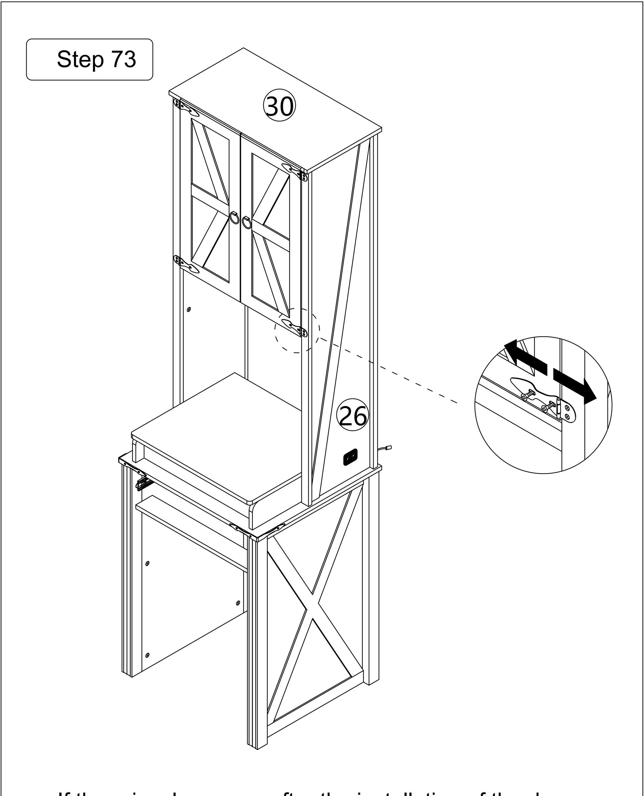
If there is a large gap after the installation of the door, please twist the screw of the door hinge back halfway and move the door left and right.
