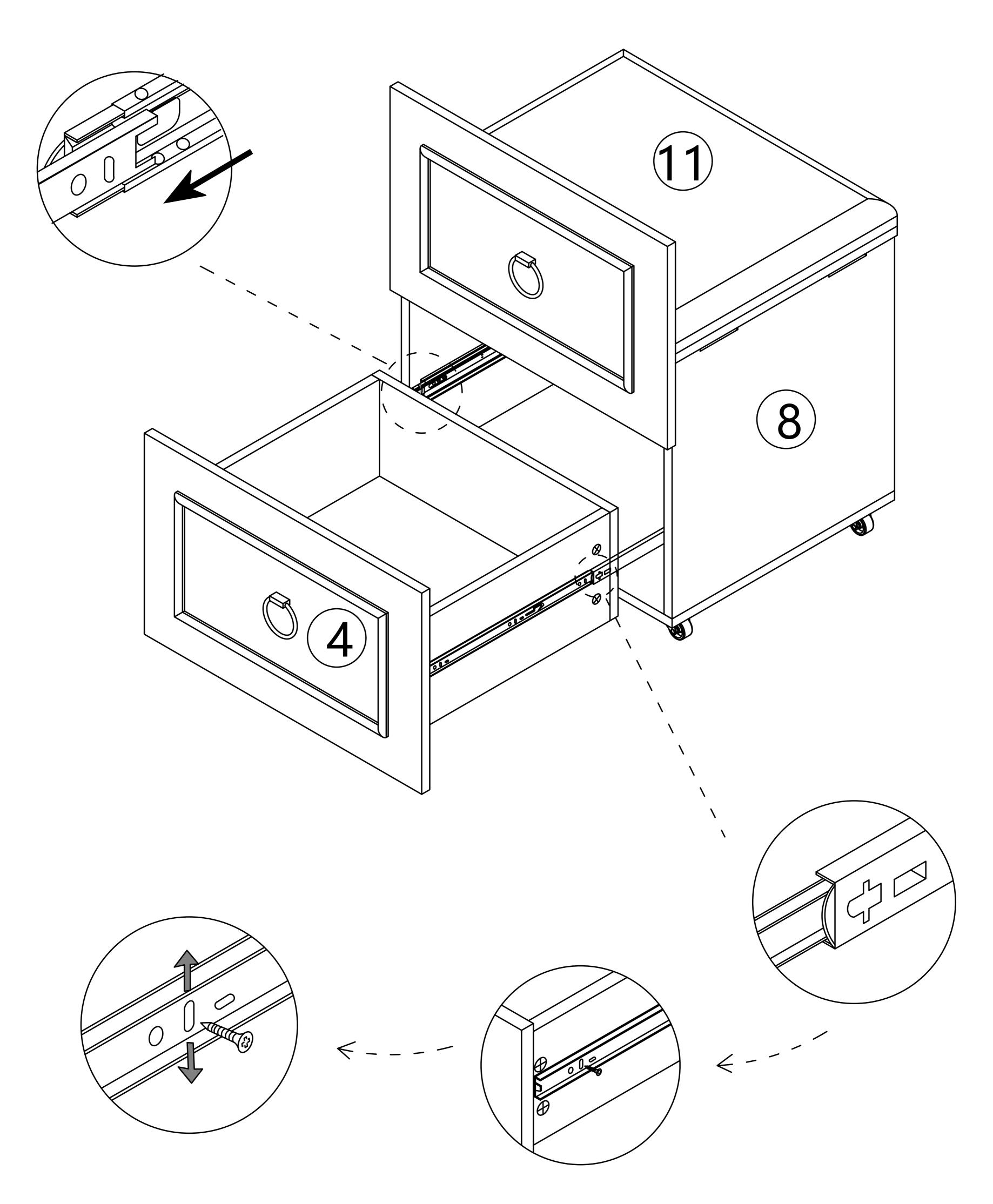
If a large gap is found after installing the drawer the slide rail can be moved up and down to adjust the gap
