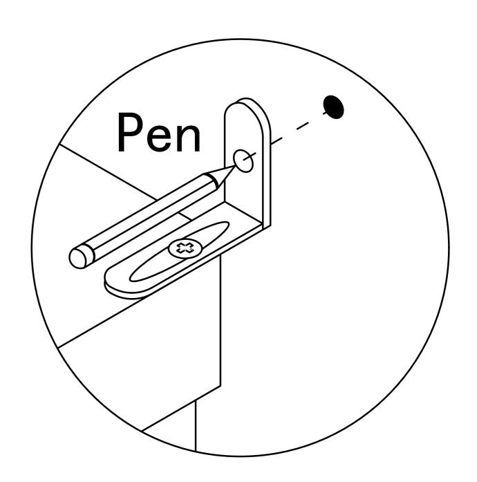
Then mark the wall with a pen through the holes in the anti-fall hardware
