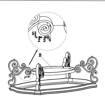
STEP 2: Attach Shelf (B) to Legs (E) by using Allen Key M4 (5), Allen Bolt 1/4" x 28mm (2) Spring Washer 1/4"(3), Flat Washer 1/4" (4)
