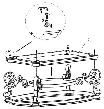
STEP 3: Attach Bottom Panel (C) to Legs (E) by using Allen Key M4 (5), Allen Bolt 1/4" x50mm(1) Spring Washer 1/4" (3), Flat Washer 1/4" (4)
