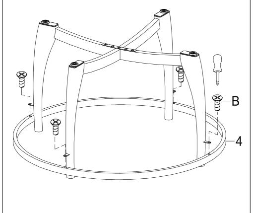
Attach top frame (4) to stretchers by using screw (B) as shown.
