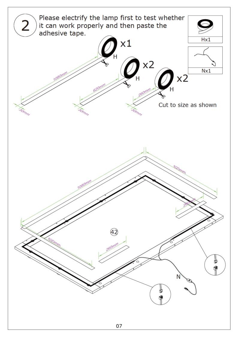
According to the actual situation, cut the tape into small sections and paste it for reinforcement
