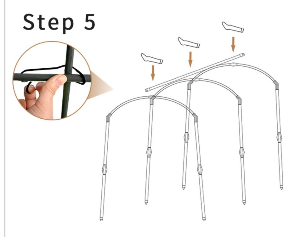
Fix the horizontal pipe in step 4 and the three arch pipes in step 3 together with a sure-clip
