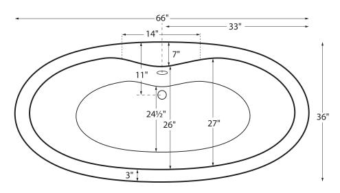
Features a 7" wide flat deck surface on the drain side for mounting faucetry.
