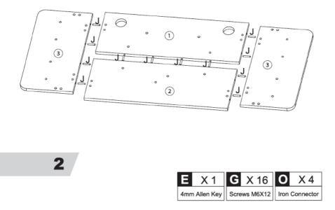
Note: The horizontal bar on the Iron Connector should be perpendicular to the seam of the table panel splice
