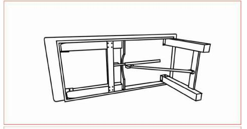
Step1:Open the box and take off the locked pins from Hole 1, then open the legs
