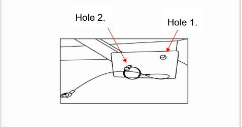
Step2: fix the pins into Hole 2.
