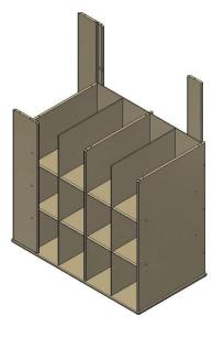
**Step 6:** Attach **Back rail and Back Brace to Left side.** Top fits into 3/8" deep groove in back rail. Notches in back brace overlap dado in left side. Tighten down halfway.
