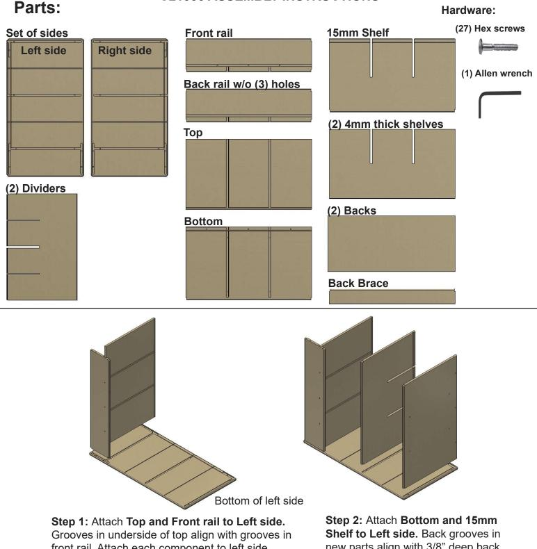
front rail. Attach each component to left side using (2) hex screws and allen wrench provided. Tighten down halfway. Back groove in top aligns with 3/8" deep back groove in left side. **Step 2:** Attach **Bottom and 15mm Shelf to Left side.** Back grooves in new parts align with 3/8" deep back groove in left side. Attach using (2) hex screws and allen wrench for each component.
