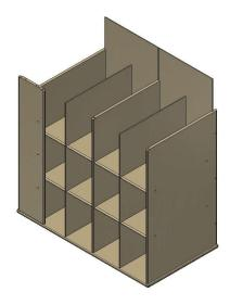
Step 4: Slide (2) Dividers into slots of all shelves and dadoes of Bottom. Attach each divider to Bottom using (2) hex screws and allen wrench. Tighten down halfway. Back face of dividers should sit flush with back face of 4mm shelves. **Step 5:** Slide in **Backs** using grooves in top, 15mm shelf, and bottom. No hardware is required in this step.
