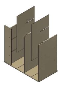
**Step 3:** Place **4mm Shelves into grooves in Left side.** No hardware is required in step. Slots in 4mm shelves align with slots in 15mm shelf.
