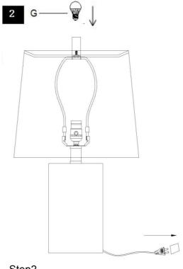
Step2 Insert the bulb(G) into the socket(C).
