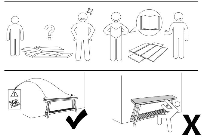
(Install tip-over restraint provided)
