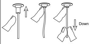
1.Using the tip of your finger or fingernail, depress the pin into the ceiling canopy, this will release the cable locking mechanism
