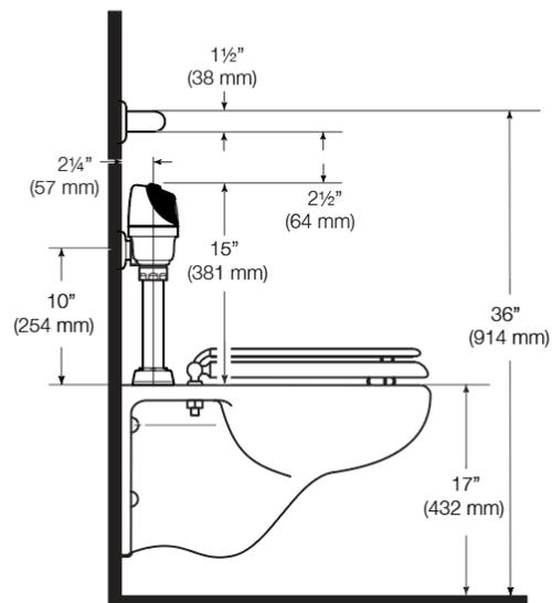
**WHEN INSTALLING IN A HANDICAP STALL:**
