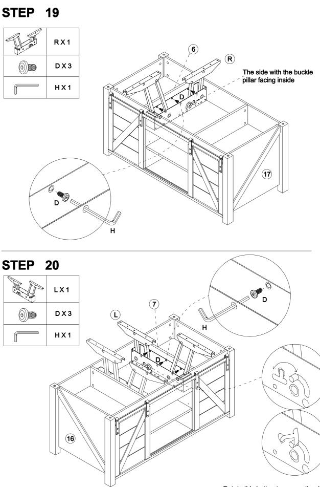
Rotate this button to secure the descent
