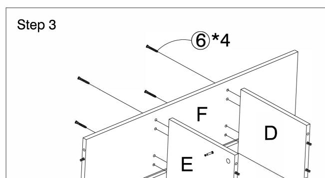
NOTE: The groove in Part F should be facing up at the back of the assembled piece.
