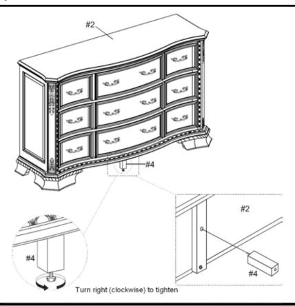
Adjust the leveler according to the ground level. To lower or to raise the center leg (#4), you need to turn the leveler clockwise or counterclockwise, respectively.
