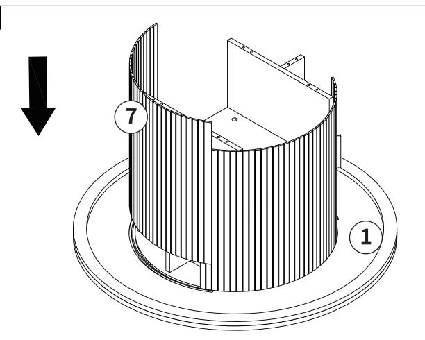
Place (7) on the outer groove on (1) as displayed.
