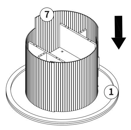
Place (7) on the outer groove on (1) as displayed.
