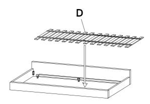
3 ATTACHED SLATS FOR DAYBED(D), WITH SELF-TAPPING SCREW(H).
