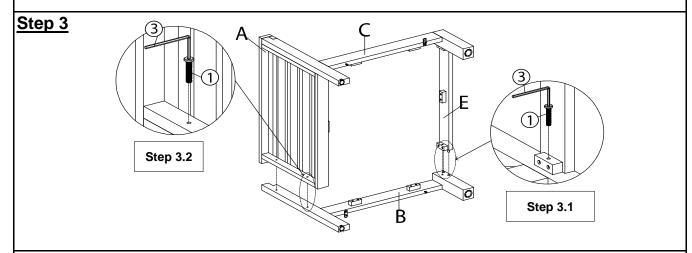
Place Left Arm Panel (B) onto the assembled frame from Step 2 Step 3.1: Align the dowels of Support Bar (E) into the positions in the Left Arm Panel (B).
