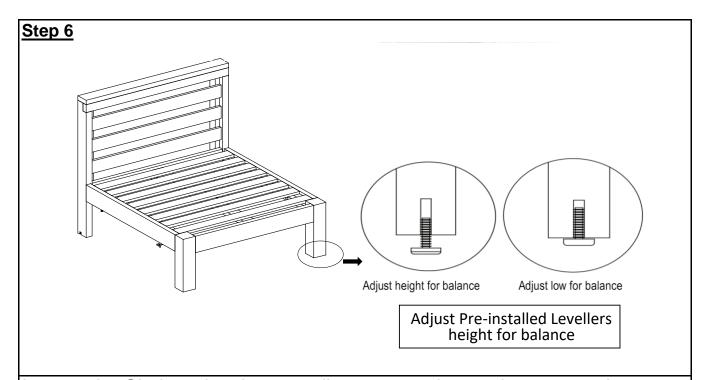
Inspect the Chair and make sure all parts are adequately connected. In a sequential manner, tighten all Screws and Bolts at all joints. With assistance from your adult partners, adjust the Levellers to desired height to avoid wobbles.
