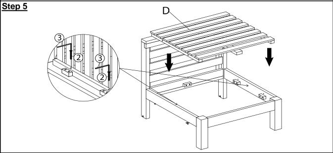
Attach the Seat Panel (D) into the Chair as shown in picture above. Affix Seat Panel (D) with Corner Chair by using Screws (2) and Allen Key (3).
